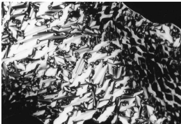
Figure 2. Fan-shaped SmA texture of 5,6-dideoxy-6-C-perfluorooctyl-D-xylo-hexanose 6 , 119°C, on cooling; 16-fold enhancement.
